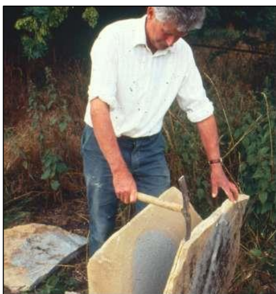
Cliving Collyweston slate (courtesy Stone Roofing Association)
